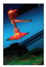
PDR's process involves pre-heating the PCB from below with a back heater and then heating the component from above. This reduces the time and energy required for topside heating, thereby minimising the potential for damage to the component, the PCB or adjacent devices. PDR's closedloop temperature monitoring system, with a non-contact IR sensor, makes the process highly controllable and repeatable, producing high quality solder joints every time.
